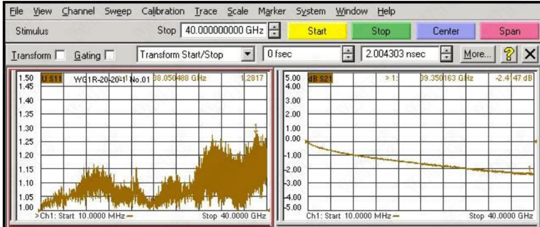
Typical Test rest results with 1 M length
