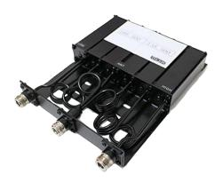
Compact duplexer 6MC150-30 is meant to provide frequency isolation between transmitting and receiving channels. Combining small geometry with low loss and close frequency spacing with selective pass characteristics this duplexer is ideal for use in systems with low-to-medium power repeaters where small physical dimensions of equipment are critical.
